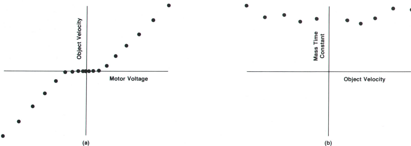
Fig. 3. A software package for the 9825S Computer is under development that will help the user determine and implement the optimum gain for a position control system. The first step is discrete characterization of the process to be controlled. This is done by plotting a series of measured data points as shown here.
