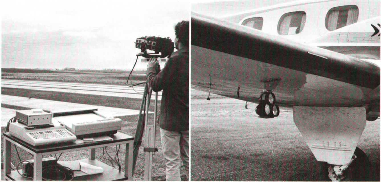
Fig. 13. Equipment used to measure the velocity of an airplane. The 3850A was an experimental model modified to produce an audible tone when pointed at the retroreflectors. The fixture holding the 3850A was also a special experimental model. (a) Experimental dynamic monitoring system. (b) Mounting of retroreflectors on the aircraft's wing.
