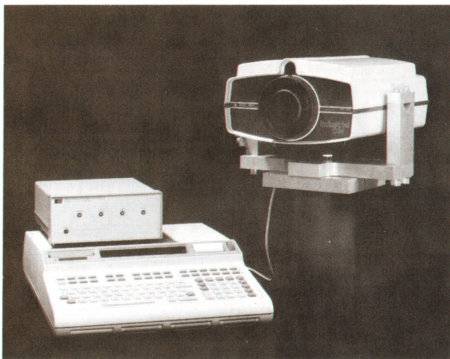
Fig. 4. This basic dynamic measurement system can be used for measurements on moving or static targets. For industrial position control applications a digital-to-analog converter or relay actuator may be added.
